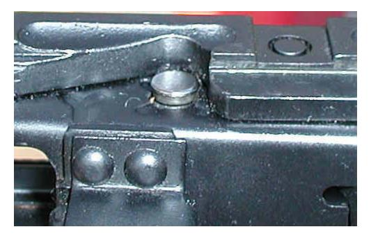
If you're just replacing the hammer you can take it out without taking out the trigger group. Just twist it in the receiver at a 90 degree angle and pop it out. It does take a bit of pressure to do so, but you won't hurt anything.
