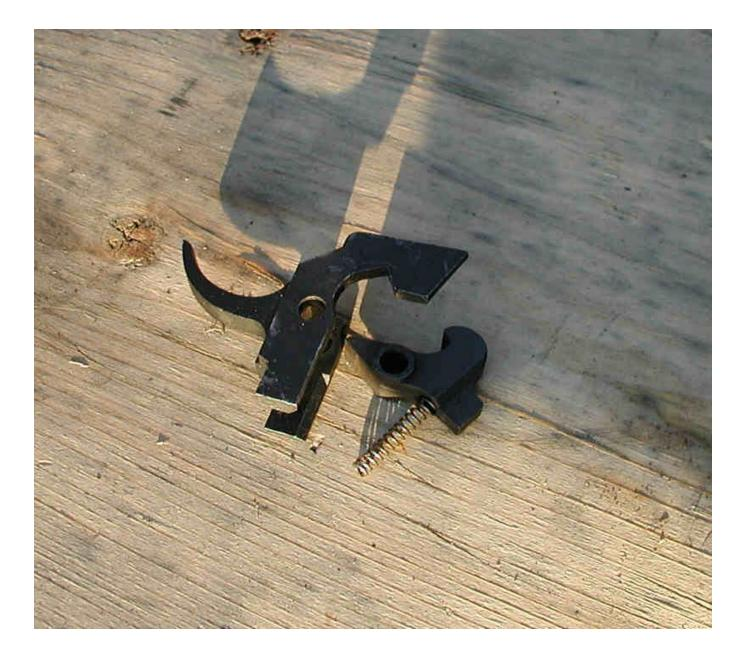
OK, here we get into the meat of the situation, putting all this crap back in. First thing I do is install the hammer, then, like above, install the Sheppard hook around the pivot pin. It helps to take a flat blade screwdriver and push the hammer spring to the side a bit to get the hook around the pin.
