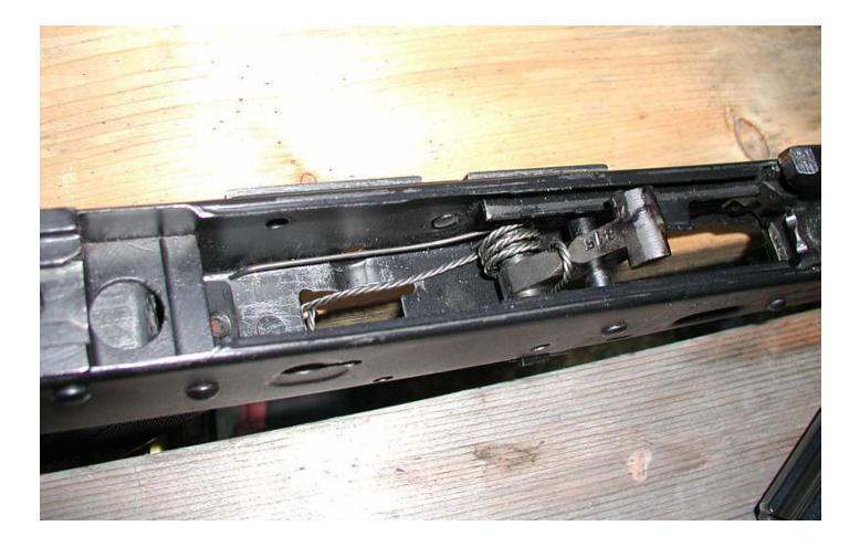
This picture is KEY to getting together a AK trigger group without a lot of cussing, bitching, and griping. When you put in the trigger pivot pin, make sure you put it in ABOVE the Sheppard hook and below the hammer spring leg as shown. Putting in the Sheppard hook is the biggest hassle for most people. Doing it this way removes that hassle.
