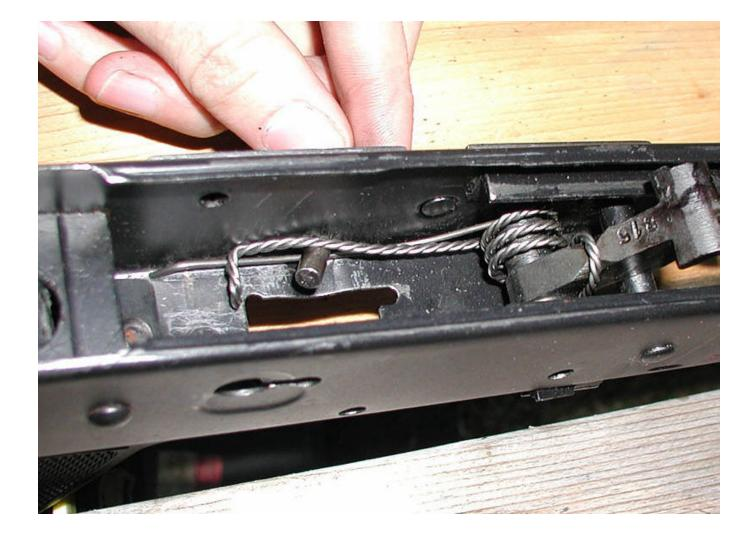
When you install the trigger group, put the disconnector, spring, and trigger together and try to line them up before putting them in the AK. Keep a finger on the disconnector pushing it down into the trigger well, so that the spring won't come out. Push the pivot pin in, lining up the trigger, disconnector, and pivot pin hole on the other side of the receiver.
