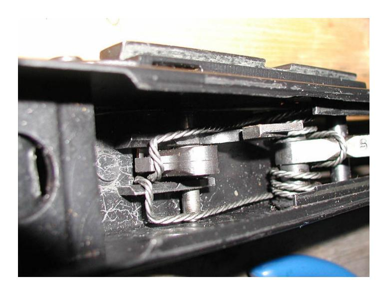
OK, last step! Done with that beer yet? Use a flat headed screw driver, (you don't need a rusty one like mine) and push the Sheppard hook over to the left side of the receiver and down. Make sure that the Sheppard hook is in the retaining ring on the underside of the pin. This keeps the trigger pin from walking out of the receiver, especially when you're firing!
