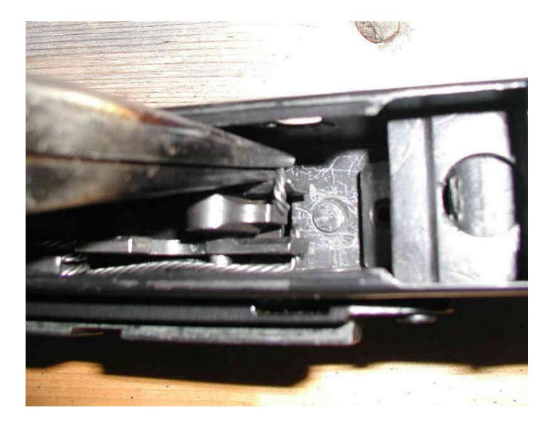
OK, almost done! Before the last step of putting the Sheppard hook in the retaining ring of the trigger pin, it helps the move the left hammer spring leg over to give you some working room. Hooking it over the disconnector will keep it in place until you need to move it back.
