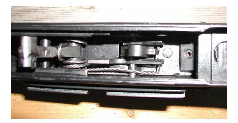
As you can see here, the trigger group is in, and the pin is inserted all the way. Use a pair of needle nose pliers to put the legs of the hammer spring on top of the left and right sides of the trigger. The legs of the hammer spring are what push the hammer forward after you pull the trigger.
