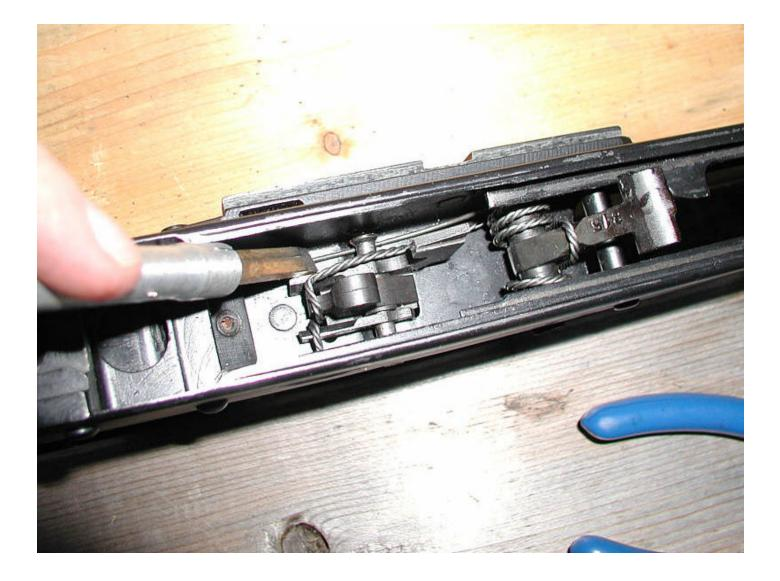
OK, your done! Feel better now? Basically this picture just shows a completed install. Notice the Sheppard hook is retaining both pins, and the hammer spring legs are correctly hooked around the bottom of the trigger. Now that you're done you can have a second beer!
