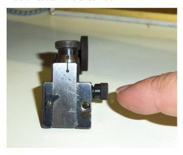
As it was explained to me, the lock bolt serves as a quick release of the Slide to make for fast and gross adjustments. You will turn it to the left until stops and then press the spring-loaded knob.
