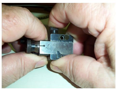
It is not an easy task. It is a strong spring and the slide does not move easy with its tight tolerances and probably years of old lubricant.
